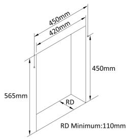
Carefully mark out the fixing screw positions as above, fit two pan head screws leaving approximately 2mm between the wall/panel and the underside of the screw head. Lift the fire into position so the keyhole slots locate on the screw heads.
